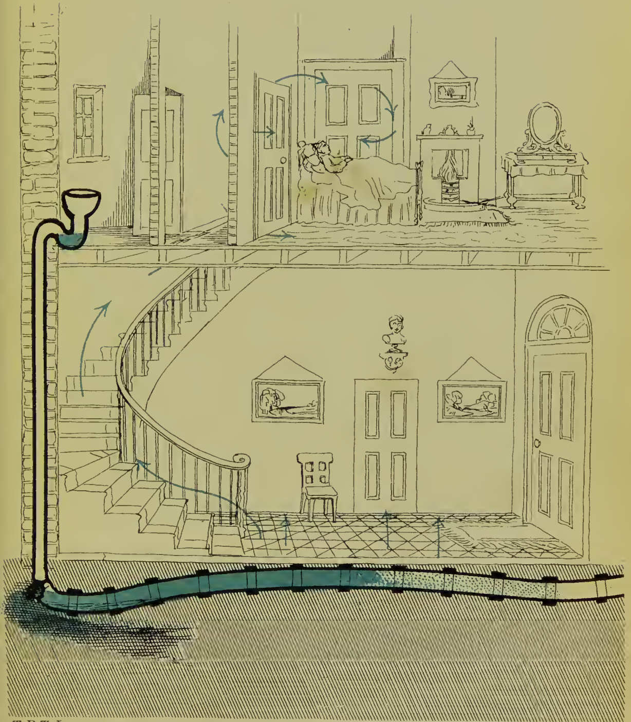
Drain under floor, with fall the wrong way. Broken pipe at the junction with fall pipe.
